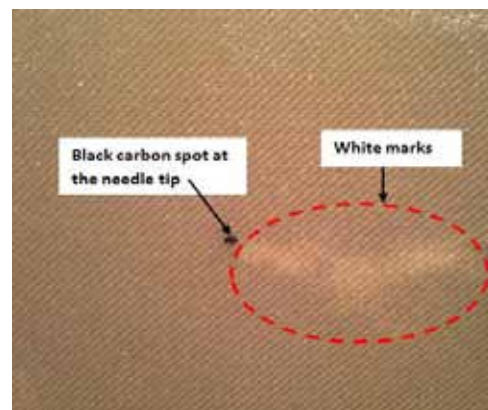
Figure 6: An example of a pressboard sample exposed to 3 hour surface discharge ageing showing the white track marks.
