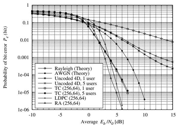
Figure 10: Multipath performance comparison of (256, 64) coding schemes
