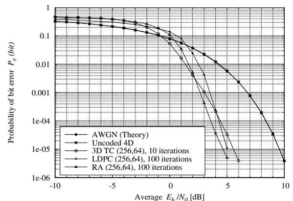
Figure 9: AWGN performance comparison of (256, 64) coding schemes
