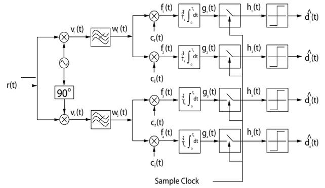
Figure 2: Four dimensional DSSS receiver structure
