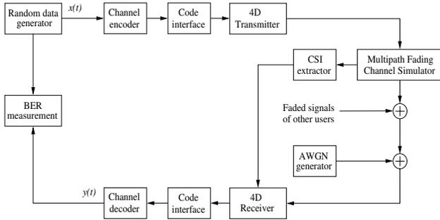
Figure 6: Coded simulation platform
